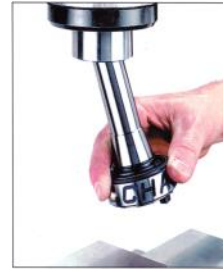
1. Load R8 Master holder to machine spindle and set collar to open position.
