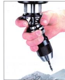
3. Remove tool with one hand by twisting collar to release tool
